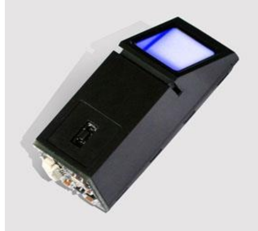
Fig 2. Fingerprint sensor SM630
